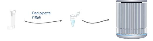
For each test you will require a negative control. Instead of DNA, water is used. This sample should typically prove negative thus proving that all of your positive samples really are positive.
