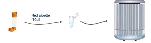
For every reaction to be run, use the red pipette to add 10µl of your C.estertheticum reaction mix to every tube.
