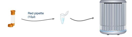
For every reaction to be run, use the red pipette to add 10µl of your C.fetus reaction mix to every tube.
