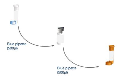
Use the blue pipette to transfer 500µl\* of the oasig Master Mix resuspension buffer into the tube of lyophilised oasig Master Mix and mix well by gently swirling. Then transfer all of that master mix into the brown tube labelled C.fetus primers/probe.
