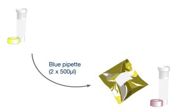
Use the blue pipette to transfer  $1000\mu$ l (2 x  $500\mu$ l) of template preparation buffer into each of the positive control template tubes. Cap and shake tube to mix.
