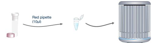
Take great care when setting up your positive control. The positive control template has the potential to give you a false positive signal in your other samples. Set positive controls up last after all other sample tubes are closed. Always change pipette tips between samples. You may even choose to set up positive controls in a separate room.
