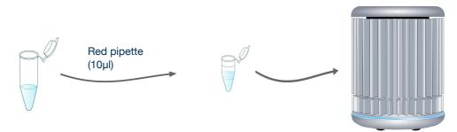
For each sample you wish to analyse, use the red pipette to add 10µl of your DNA sample to the required reaction tubes. Close these tubes after adding the sample. Always change pipette tips between samples.
