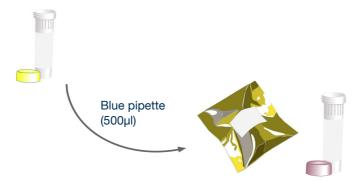
Use the blue pipette to transfer 500µl of template preparation buffer into the positive control template tube. Cap and shake tube to mix.
