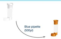
Then use the blue pipette to transfer 500µl of water into the brown tube labelled FMDV primers/probe. Cap and shake tube to mix. A thorough shake is essential to ensure that all components are resuspended. Failure to mix well can produce poor kit performance.
