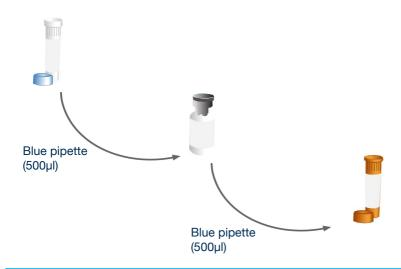
Use the blue pipette to transfer 500µl\* of the oasig Master Mix resuspension buffer into the tube of lyophilised oasig Master Mix and mix well by gently swirling. Then transfer all of that master mix into the brown tube labelled HSV1&2 primers/probe.
