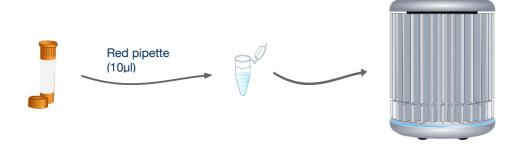
For every reaction to be run, use the red pipette to add 10µl of your HSV1&2 reaction mix to every tube.
