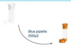
Then use the blue pipette to transfer 500µl of water into the brown tube labelled HTLV-2 primers/probe. Cap and shake tube to mix. A thorough shake is essential to ensure that all components are resuspended. Failure to mix well can produce poor kit performance.
