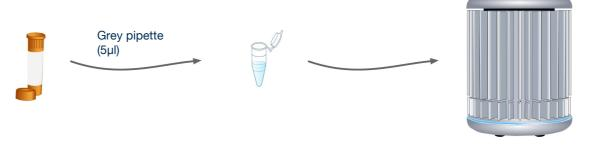
For every reaction to be run, use the grey pipette to add 5µl of your ISAV-EU primers/probe mix to every tube.
