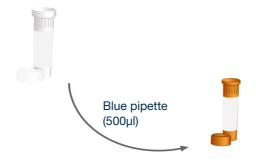
Then use the blue pipette to transfer 500µl of water into the brown tube labelled ISAV-EU primers/probe. Cap and shake tube to mix. A thorough shake is essential to ensure that all components are resuspended. Failure to mix well can produce poor kit performance.
