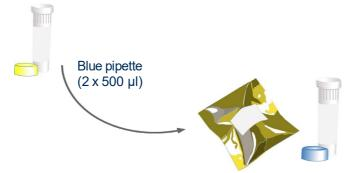
Use the blue pipette to transfer 1000  $\mu$ l (2 x 500  $\mu$ l) of template preparation buffer into the Internal Extraction Control DNA tube. Cap and shake tube to mix.
