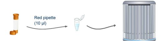
For every reaction to be run, use the red pipette to add 10 µl of your *B. bronchiseptica* reaction mix to every tube.
