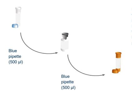
Use the blue pipette to transfer 500  $\mu$ l\* of the oasig Master Mix resuspension buffer into the tube of lyophilised oasig Master Mix and mix well by gently swirling. Then transfer all of that master mix into the brown tube labelled *B. bronchiseptica* primers/probe.
