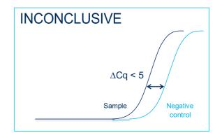
If the sample amplifies < 5 Cq earlier than the negative control, then the positive sample result is invalidated, and the result should be inconclusive determined due to test contamination. The test for this sample should be repeated.
