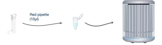
For each test you will require a negative control. Instead of DNA, water is used. This sample should prove negative thus proving that all of your positive samples really are positive.
