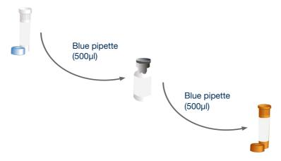
Use the blue pipette to transfer 500µl\* of the oasig Master Mix resuspension buffer into the tube of lyophilised oasig Master Mix and mix well by gently swirling. Then transfer all of that master mix into the brown tube labelled Goat primers/probe.
